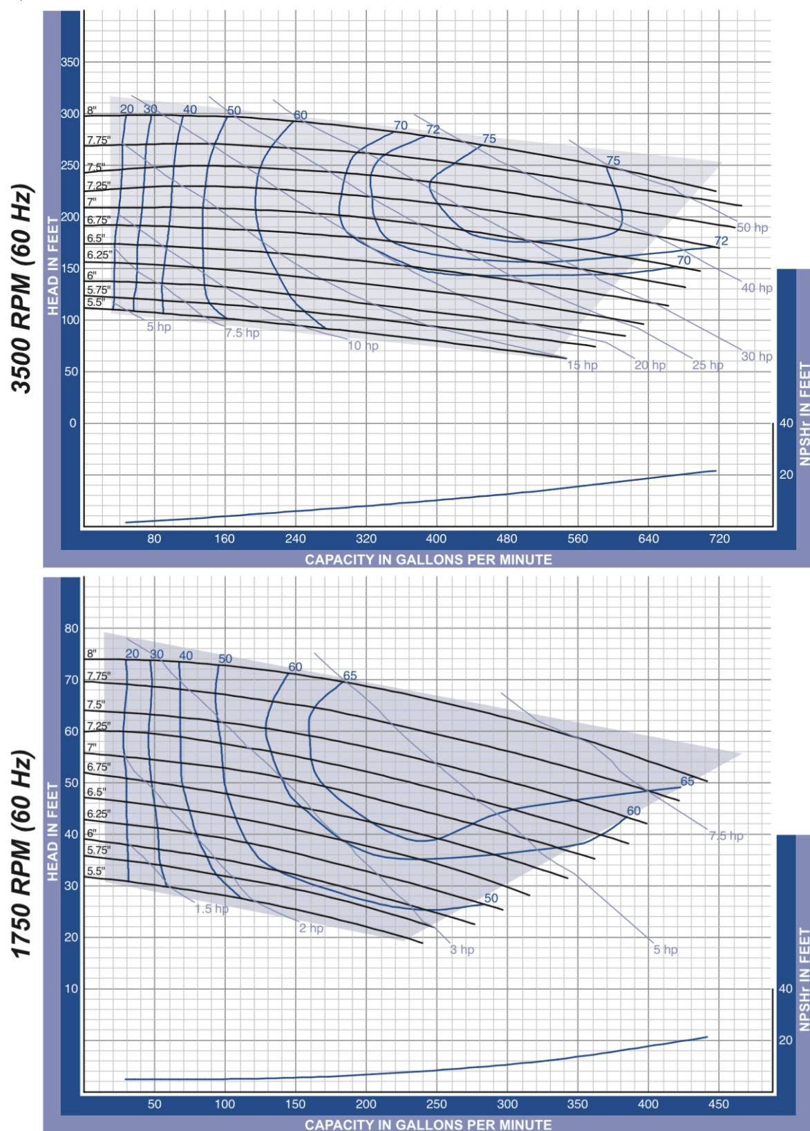
The curves are based testing water at 70° F and have a tolerance of  $\pm 5\%$  applicable to all of them. For different operation conditions please contact us. The impeller diameter is in inches.
