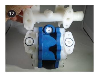
3 Stand the pump upright onto the suction manifold feet (item 12). Press the valve balls (item 15), valve seats (item 14), and seat o-rings (item 13) into the discharge manifold (item 16) in the same order as the suction side was done in step 11. Place the discharge manifold atop the pump, tighten, and torque the discharge manifold bolts (item 11) in an "X" pattern. Torque to 50 in-lbs (5.6 N-m).
