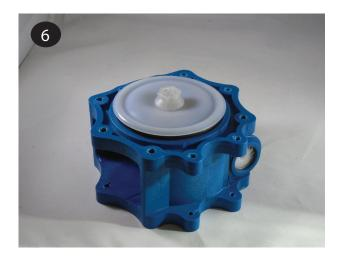
The other diaphragm(s) (item 17) and inner/outer plates (items 19 & 23) can be installed onto the opposite end of the shaft (item 27). It may be easier to thread the molded in bolt into the shaft if the diaphragm(s) is inverted on one or both sides. This can be done by hand.
